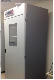
Incubator holding 800–1,000 seeded trays can produce ~1 kg crude protein overnight
